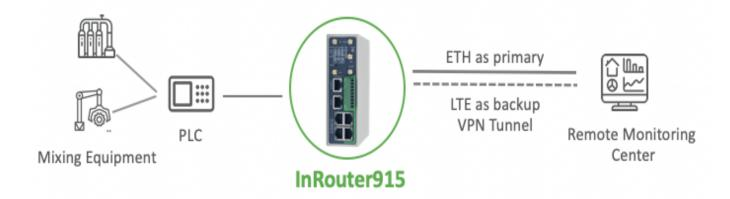
The monitoring system of concrete mixing equipment consists PLC, edge computing gateway InRouter915 and cloud monitoring center.
